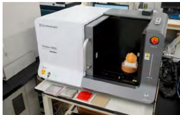
Shimadzu Corporation's XSeeker X-ray CT system: a desktop-sized device that makes it easy to scan food samples
