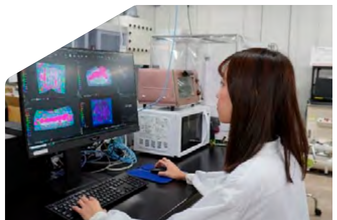
The process of quantifying and analysing internal food data captured by CT using the dedicated software 'VGSTUDIO MAX'
